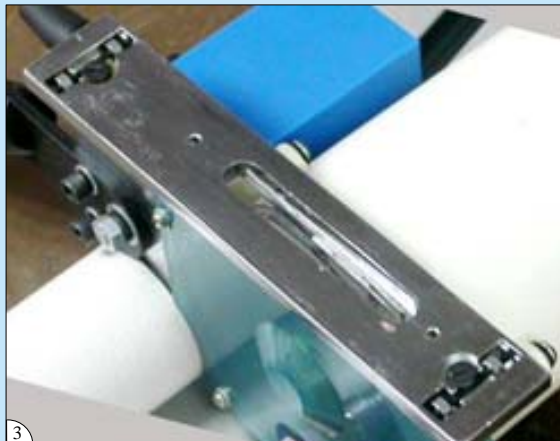
3 配備微型軸承，操作輕鬆自如 Fitted with mini-bearing for easy operation
