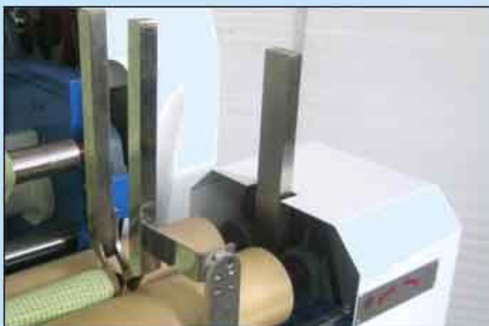
捲布擋板,能降低捲布時布卷左右擺動的范围 Cloth stopper reduce swing of fabric roll
