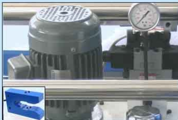
備有油壓式對邊裝置及對邊電眼,自動追蹤對邊,使布邊平整美觀 Equipped with hydraulic edge alignment device and edge alignment electric eye, automatic alignment for neat fabric edge
