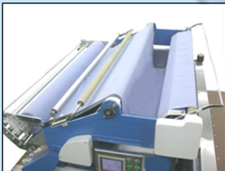
“U”型松布功能，無張力拉布 “U” Type Fabric Loosening for Tension Free Cloth Laying
