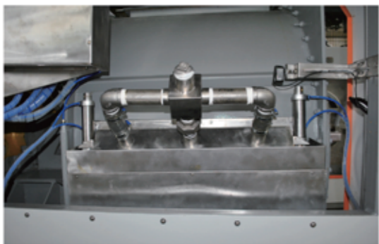
氣動排毛頭裝置 Pneumatic foam removal device
