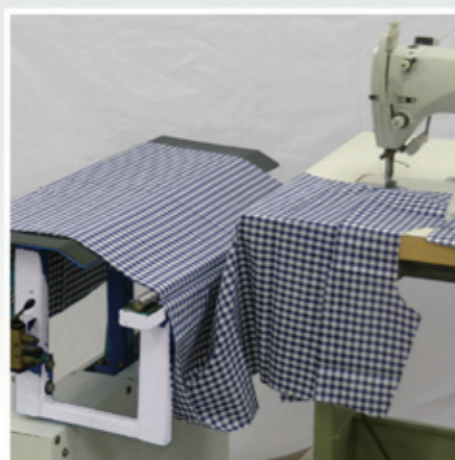
NS-6020工作時，裁片夾可調至與衣車同步令車縫時更順暢，完成後自動回位 In operation, cutting pieces clip can be adjusted in the same pace with stitch machine, make stitch smooth, after finish it will restore automatically
