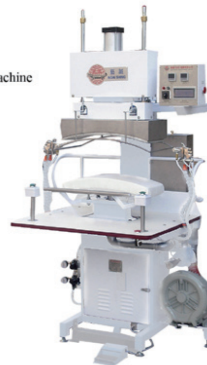
NS-8410P 特別設計模，配合不同恤衫領面 Special designed mould for fitting for various kinds of shirt collar shape
