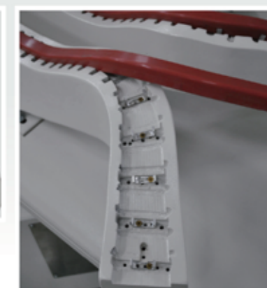
NS-9512下模硅膠條可左右微調 Silica rubber of lower mould can be adjusted right and left slightly
