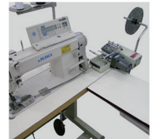
A903安裝位置圖 Appearance of A903 after being installed to a sewing machine
