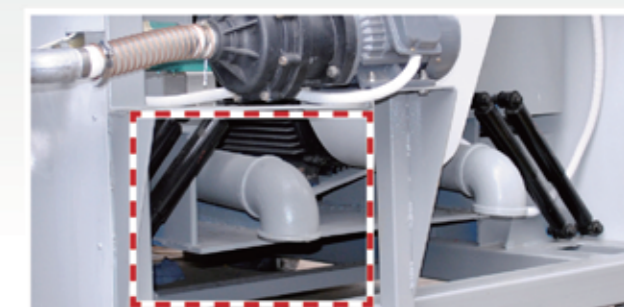
雙排水系統 Double outlet water draining system
