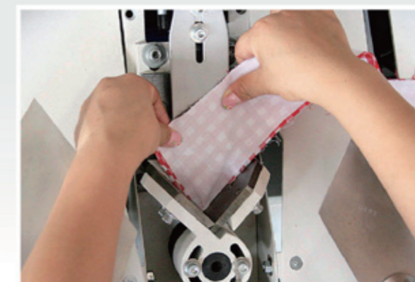
NS-81P 切領操作 Collar cutting operation
