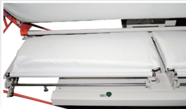
特製壓布框，可自動拉展褲管 Special fabric clamping frame could stretch and hold trousers' legs automatically so as to get a better pressing effect
