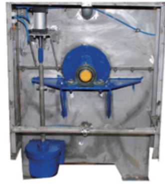
氣動排水 pneumatic water draining device
