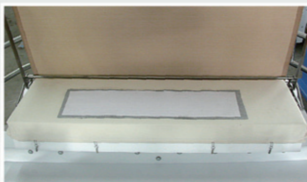
雪佛龍壓布架可將布片固定，防止旋轉時造成移位 Teflon fabric holding frame can hold the fabric in position to prevent it from moving during rotation
