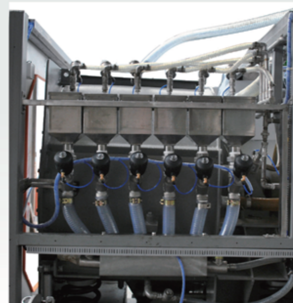
最多可選購6個5升的藥水缸 Up to six chemical dosing boxes of 5 liters volume can be purchased
