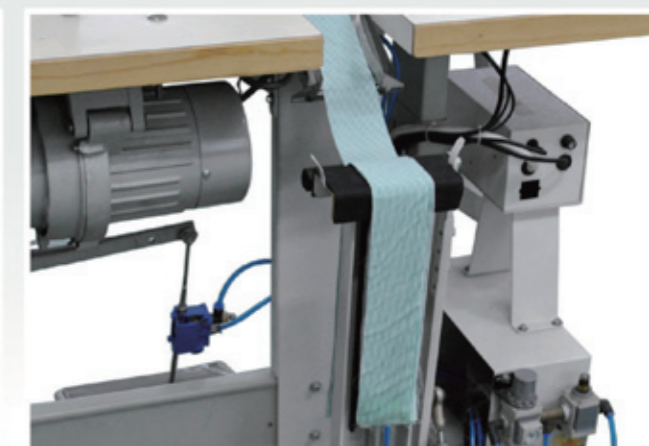
NS-94AC-1 電眼感應自動收料 Automatically material stacking by photoelectric sensing
