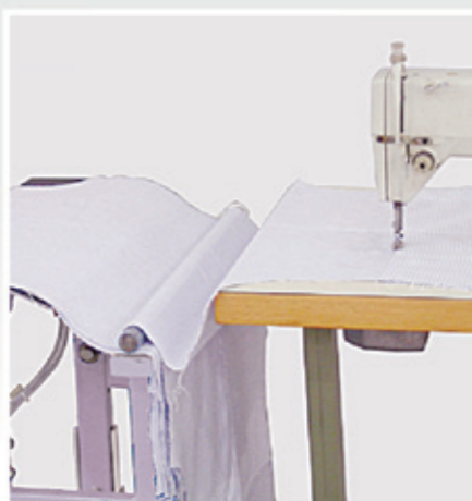
NS-6006 最適合用於恤衫擔桿及袖側 Best for shirt yoke and sleeve placket
