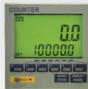
NS-58/NS-59電子計數布碼表，記錄布匹長度 Equipped with electronic meter for recording cloth winding length
