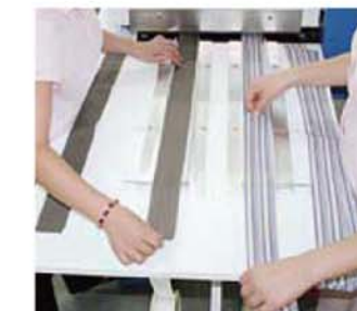
NS-5601 粘褲襠 Waistband and tape fusing
