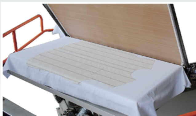
NS-8933/NS-8934 壓前幅 Pressing shirt front
