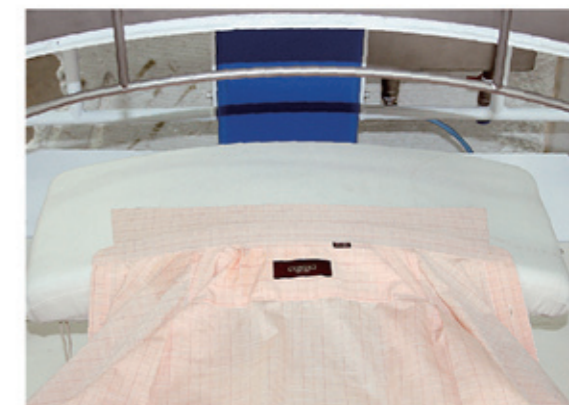
NS-8410P 特別設計模，配合不同恤衫領面 Special designed mould for fitting for various kinds of shirt collar shape
