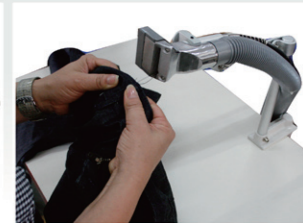
NS-3110自動剪線及吸線頭 Thread trimming and sucking
